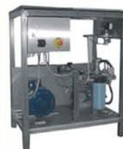
6 HP waterpump provided with: - junction box - controller box - water supply - compressed air supply
